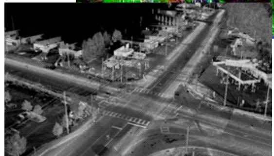
Our state-of-the-art technology equipment from ViaTech, Norway -ViaPPS Mobile Lidar system is equipped with High precision 360 degree laser scanner, inertial measurement , GNSS equipment, 360 degree rotatable Ladybug digital cameras, and Odometer etc. that can be adjusted to meet specifications of individual projects.
